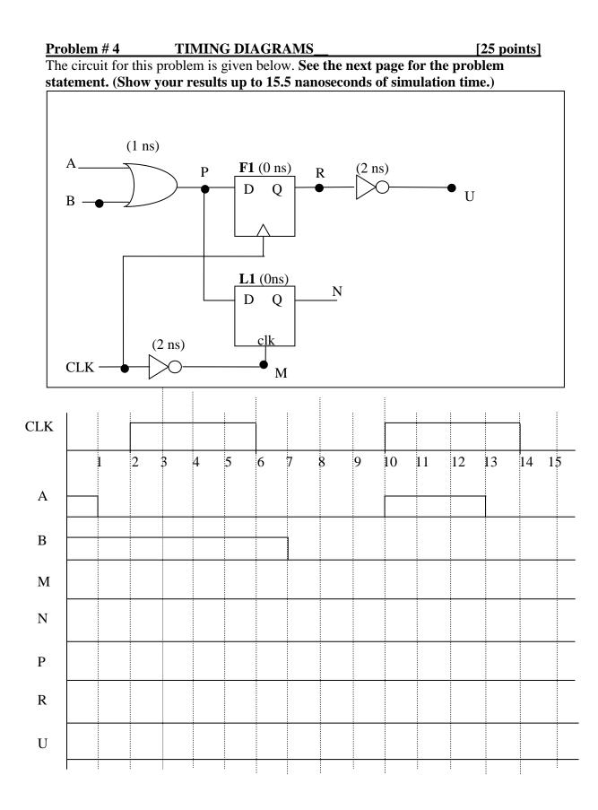
In this circuit, L1 is a positive level-sensitive D latch.
