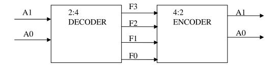
That is, the encoder takes the output of the 2:4 decoder and must produce the original input into the decoder.
