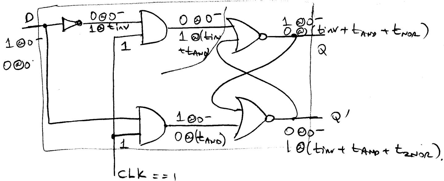
$\therefore Q'$  becomes stable  $@(t_{INV} + t_{AND} + 2 t_{NOR})$
