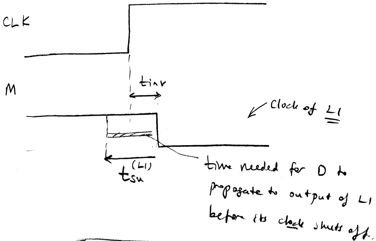
$$\therefore t_{su}^{(ff)} = t_{su}^{(L1)} - t_{inv} \quad (= t_{inv} + t_{prop} + 2t_{ROR} - t_{inv})$$
