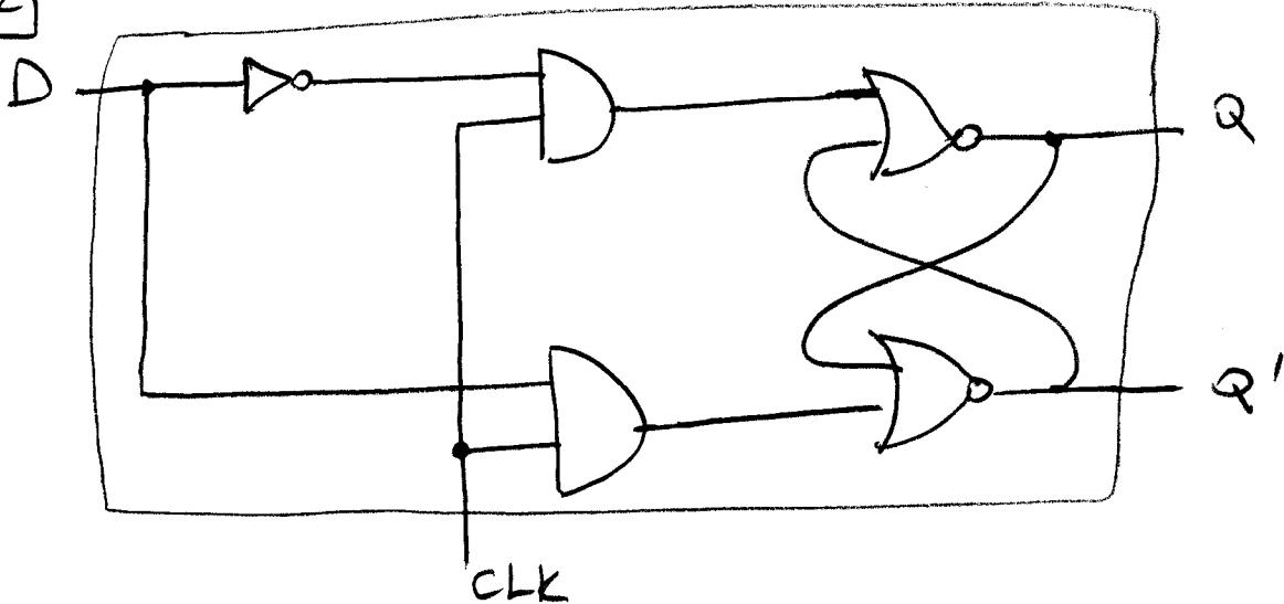
Ⓐ D-to-Q delay: max. delay incurred from a change in D (all other inputs are held constant) to a stable Q and  $Q'$ .
