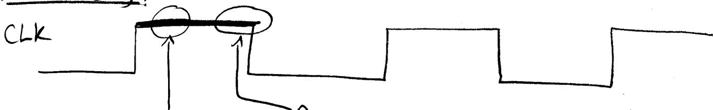
D-to-2 delay irrelevant here since, there is plenty of time remaining to copy D to Q.
