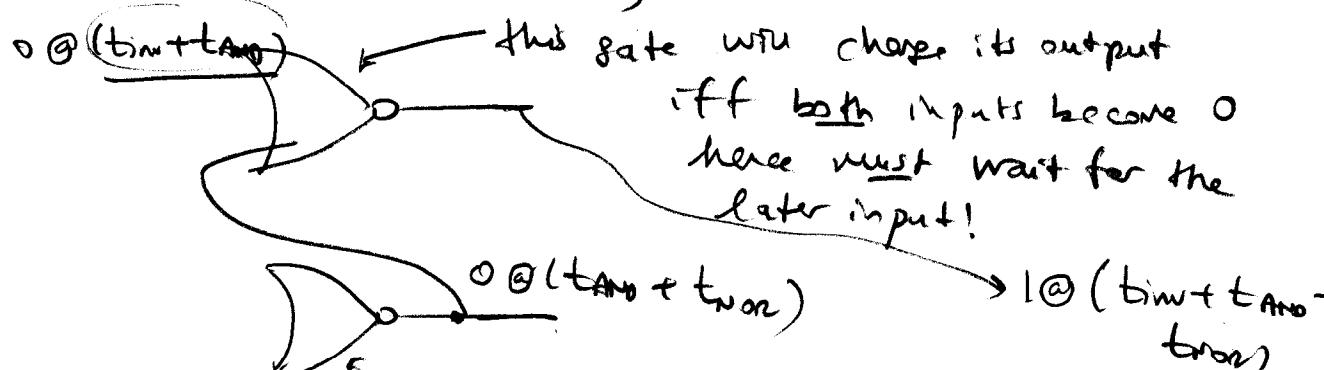
then  $Q'$  'stable'  $0 @ (t_{inv} + t_{AND} + t_{NOE})$
