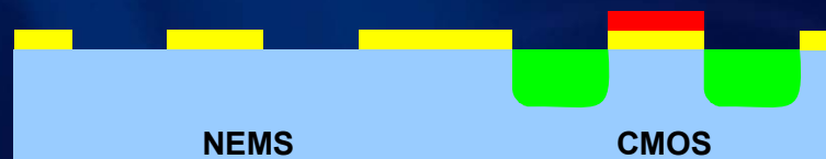
(b) Definition of active area for CMOS
