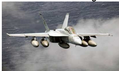
F/A-18 Hornet The first aircraft with carbon fiber wings
