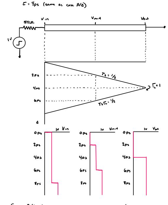
A/B has more utility since Ts = 1 and the load is matched Case to the line. In this Case, the whole Signal propagates through the line in yes. Using case B/c, To: 1/2, so the Signal is papagated in 0.5V , norement .
