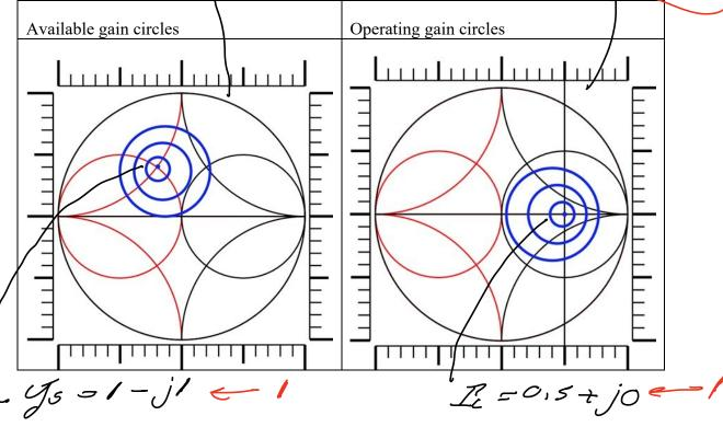
A FET in common-source mode has operating and available gain circles as shown (50 Ohm impedance normalization). Find the optimum generator and load impedances (in complex Ohms).
