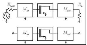
We first impedance-match the generator to the transistor input and then impedance-match the load to the transistor output (upper diagram). We then disconnect the generator and the load (lower diagram), leaving us with the transistor and its input and output networks, which we can an "amplifier".
