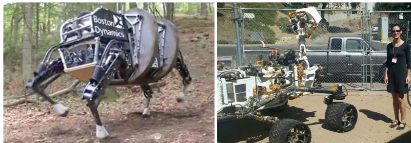
Fig. 1.4 Rough terrain mobile robots. An LS3 (Legged Squad Support System) quadruped robot (left) and an on-earth twin of the Curiosity Mars rover (right), with six articulated wheels. (The author is at right, for scale.)
