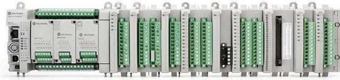
Figure: Industrial PLC with I/O modules
