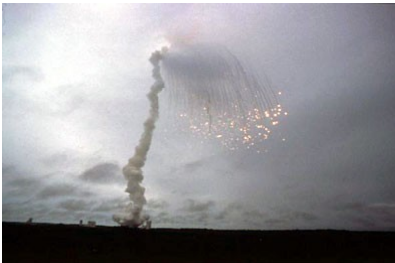
Figure 1: Ariane 5 rocket explodes in 1996 due to overflow and wraparound in 16 bit signed integer
